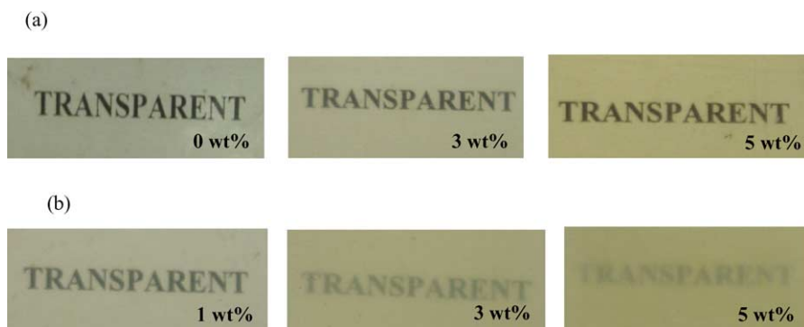
Fig. 7. Optical clarity of composites. In each case a 3 mm thick film was kept on a white paper with the word transparent written on it (a) clay 2 and (b) clay 1. Clay content is given in weight percent.
